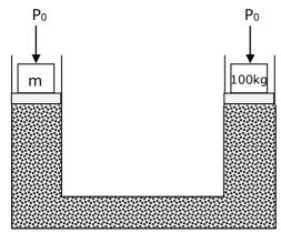
Atmospheric pressure  $\mathsf{P}_0$  will be acting on both the limbs of hydraulic lift.
